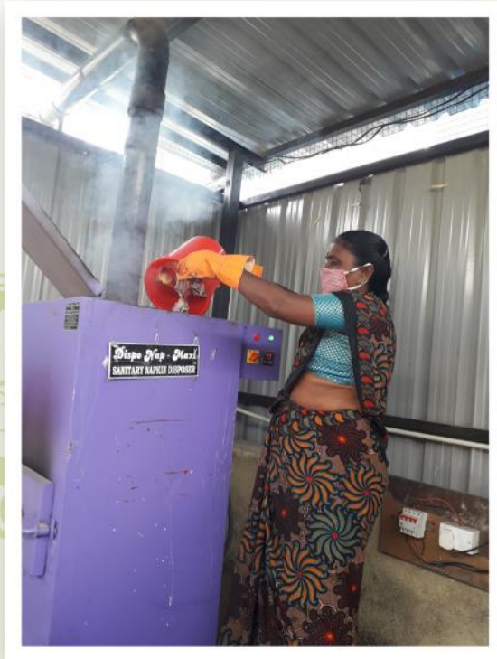
Disposal of napkins in incinerator
